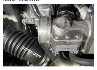
3) On the metal turbo intake, unclip and remove the large plastic breather hose:
