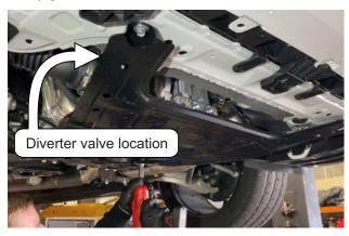
2) Loosen the hose clamp and remove the rubber intake hose:
