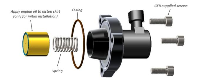
Ensure the DV+ valve body, piston, spring, and o-ring are assembled as shown above, then install the assembly onto the factory mounting location using the supplied screws, making sure to hold the piston during this process to prevent it from falling out.
