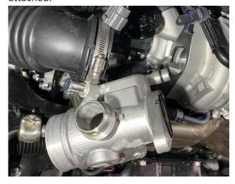
6) Unclip the electrical connector from the diverter valve, then use a T27 Torx to undo the three screws. Now remove the diverter valve:
